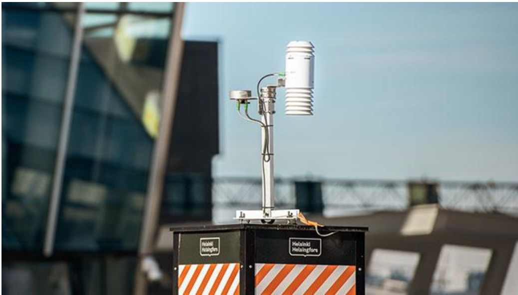
Vaisala AQT530 stationary mid-cost sensor installed in Helsinki (source: HOPE)
