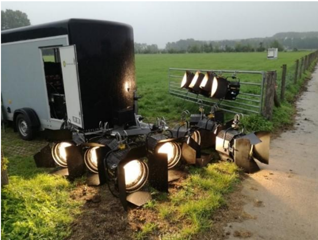
Loads connected to diesel generators, replicating the energy demand of a typical event
