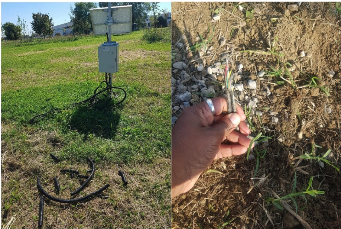
Figure 1 - Damages to the soil's monitoring system. Source: UniFE
