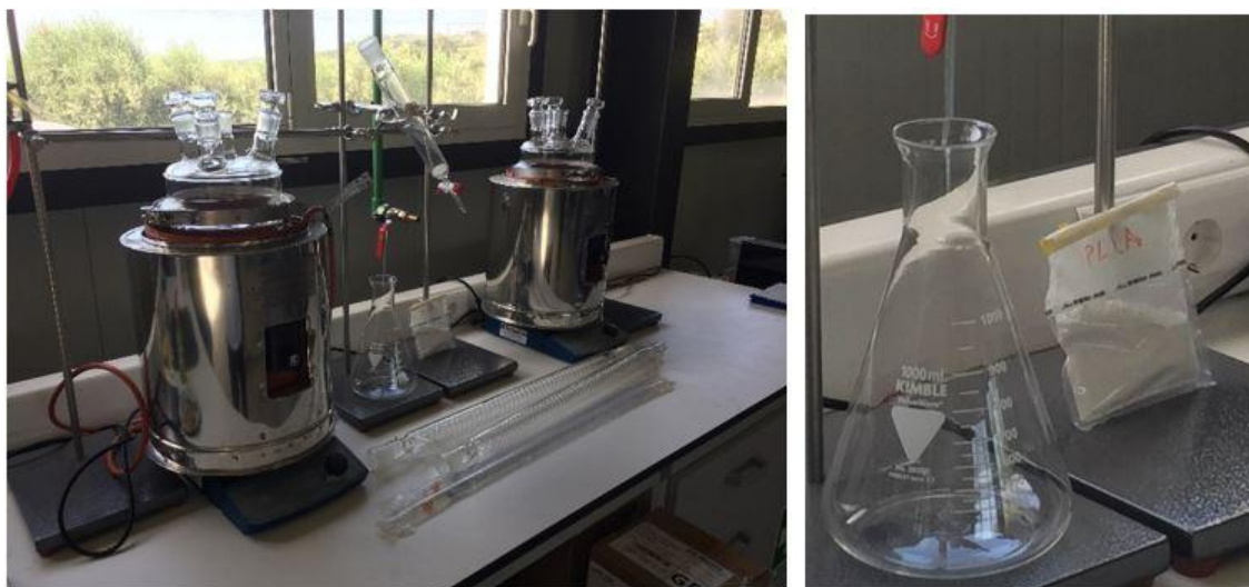
Pic.9: The polymerisation unit and the PLA product
