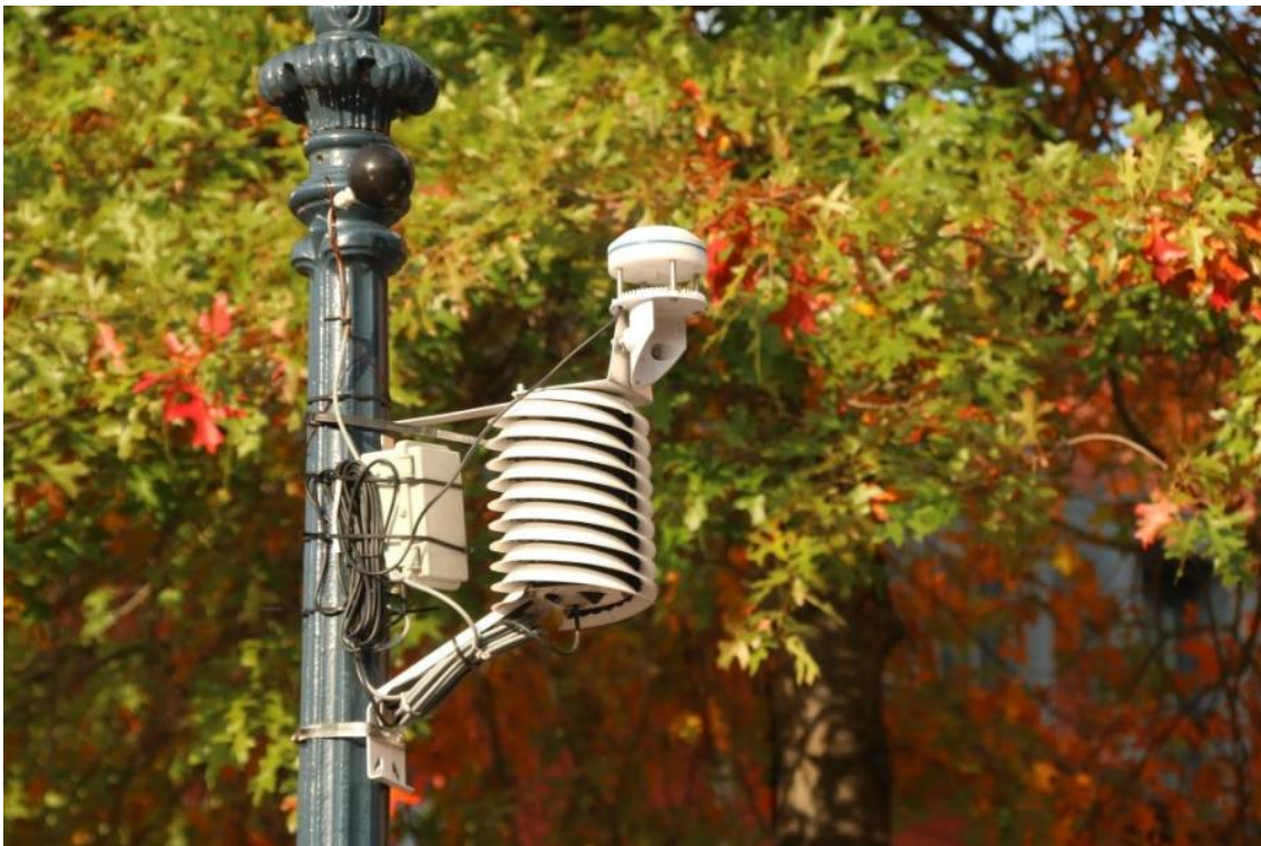
Sensor for measuring air temperature at a lamp post. Image: Birgit Georgi
