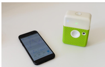
Figure 5. Small sensor designed and built by TERA, partner of the UIA DIAMS project. Mobile app shows the latest particles concentrations as measured by the user. About 2000 sensors will be made available for the DIAMS community.
