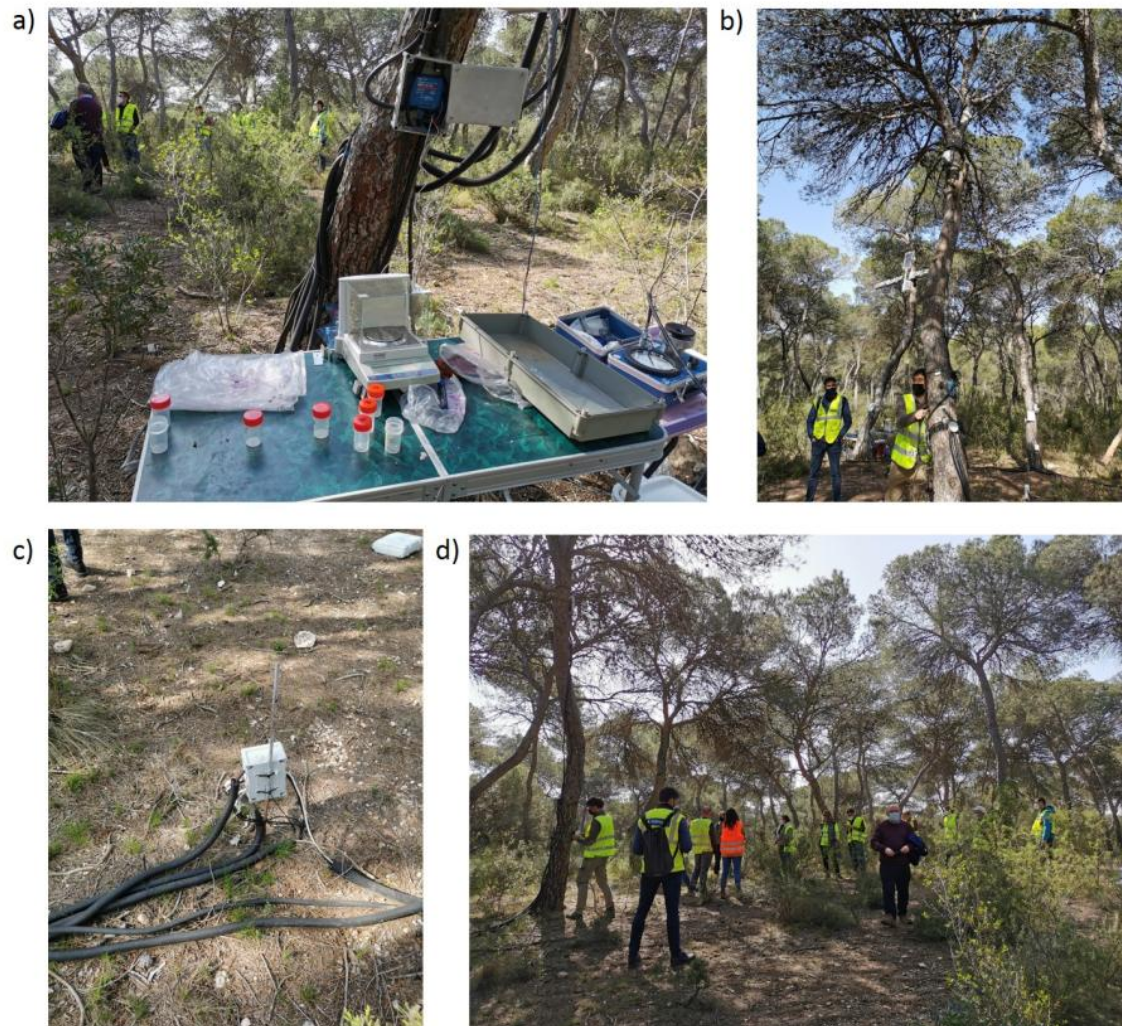
Figure 4. The experimental plot at “la Vallesa” forest: a) UPV scientists have taken their lab into the field: b) Prof. del Campo briefing visitors about the tree water activity monitoring; c) soil moisture sensors; d) visitors at “la Vallesa” experimental work.
